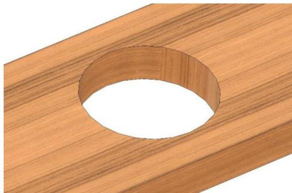
A hole is drilled in the required place on the terrace (double floor). The size of the hole depends on the type of socket, for type STAKOHOME-7702-A it is a hole approx. 170mm
