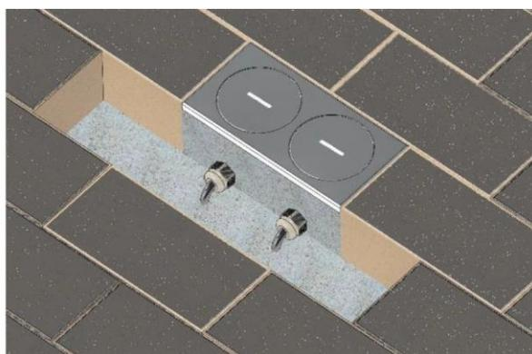
The floor box is placed in a prepared place so that it is possible to add paving (according to the shape and size of the paving). A mortar / concrete bed is prepared under the floor box and the entire floor box is fixed with concrete. Note: the flosser chooses the method of fixing / concreting the floor box (eg according to the type and height of the paving). Therefore, the installation may differ from this installation design.
